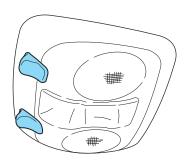
If equipped with Remote Keyless Entry, the courtesy lamp will illuminate whenever any door is opened and will remain on for 25 seconds after the door is shut or when the ignition is turned to the ON position.
